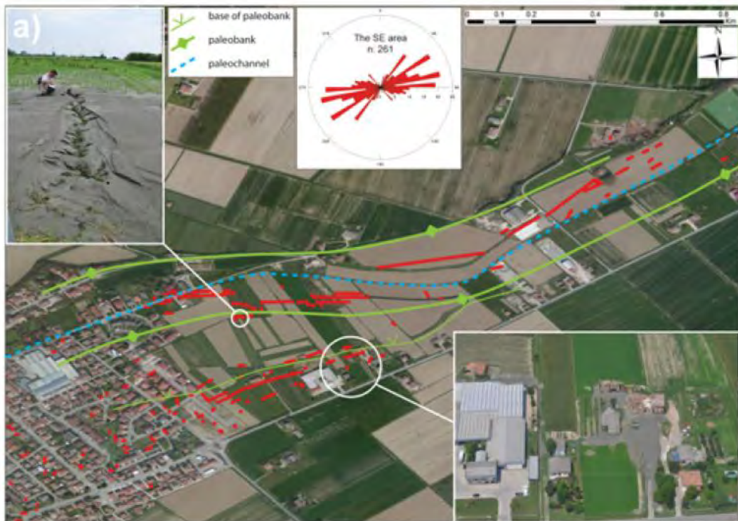
Figure 5-13 Examples of coseismic geological effects of the four study areas at different scales of observation (satellite view from Bing Maps; aerial and field view from Emergeo survey, 2013).
