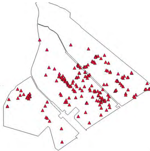
Figure 6-24 Evidences of liquefaction (sand boils and fracture) in Nakamachi (a) and map reporting the evidences of liquefaction with red triangles (b. Source Geotechnical Extreme Events Reconnaissance).
