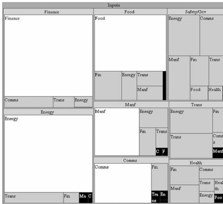
Figure 1-7: U.S. CI economic “use” interdependency. White & ¼ high-value inputs ($100 billion to a maximum value of $500 billion). Gray & ¼ medium value inputs ($10–$100 billion). Black & ¼ lower value of inputs ($1 million to $10 billion). Each sector block is proportional to the size of its total value of economic inputs consumed by the sector. Each square within each sector block indicates the proportional size of economic inputs in dollars. (Macaulay, 2009)
