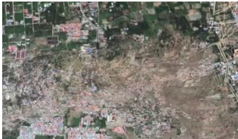
Figure 1-1: Examples of flow failure induced by seismic liquefaction in (a) Alaska (1964) and (b) Indonesia (2018).
