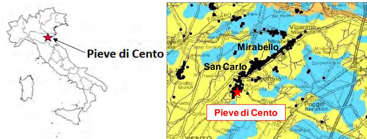
**Figure 2.97:** Location of Pieve di Cento: a) within Italy map; b) geological map of the region (in blue is represented the fine-grained deposits and in yellow sand deposits from Appenninic rivers)
