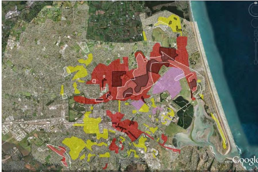
**Figure 5.38:** Liquefaction map showing the areas of liquefaction and severity observed from different earthquakes. 4th Sept 2010 (white contours), 22nd February 2011 (red, yellow, magenta areas; Cubrinovski and Taylor, 2011) and 13th June 2011 (black contours; Cubrinovski and Hughes, 2011).
