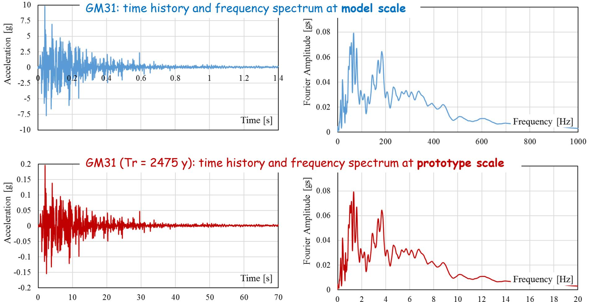
In some cases to achieve liquefaction it was necessary to amplify GM31
